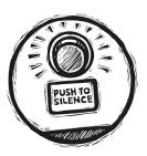
**Do** remember that the audible alarm can be silenced by pushing the lighted button located directly above the "Push to Silence" label on the front of the electrical control panel. With normal use, the tank has a reserve storage capacity good for 24-48 hours.
